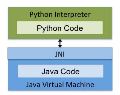
Figure 4: Communication between CPython and the Java Virtual Machine via JNI.
